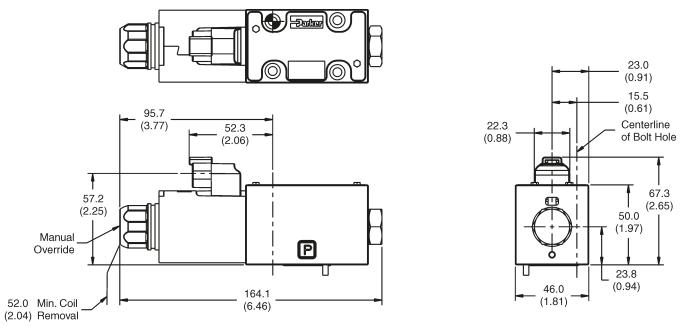
Note: 22.0 mm (0.87") from bottom of bolt hole counterbore to bottom of valve.
