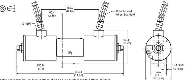
Note: 22.0 mm (0.87") from bottom of bolt hole counterbore to bottom of valve.
