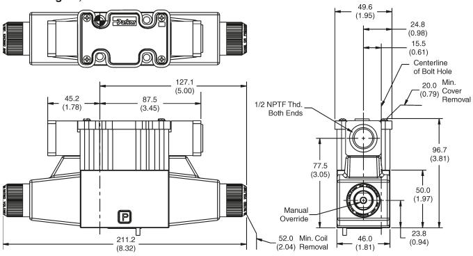
Note: 22.0 mm (0.87") from bottom of bolt hole counterbore to bottom of valve.
